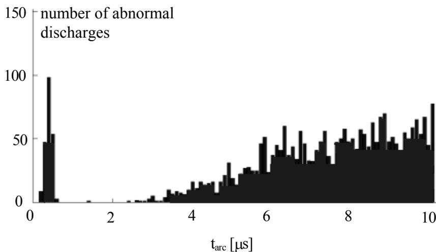
**Figure 4. Histogram of  $t_{arc}$  recorded during stable process condition**
