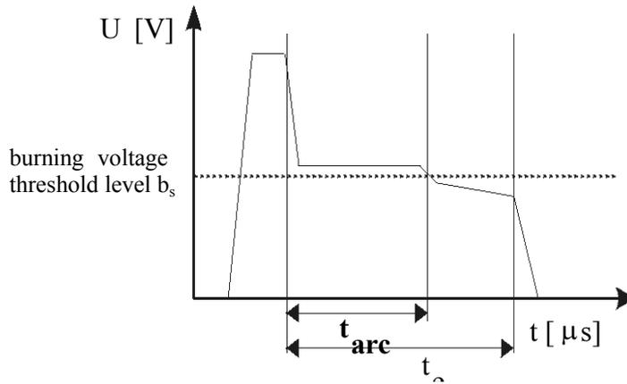
**Figure 3. Definition of  $t_{arc}$**
