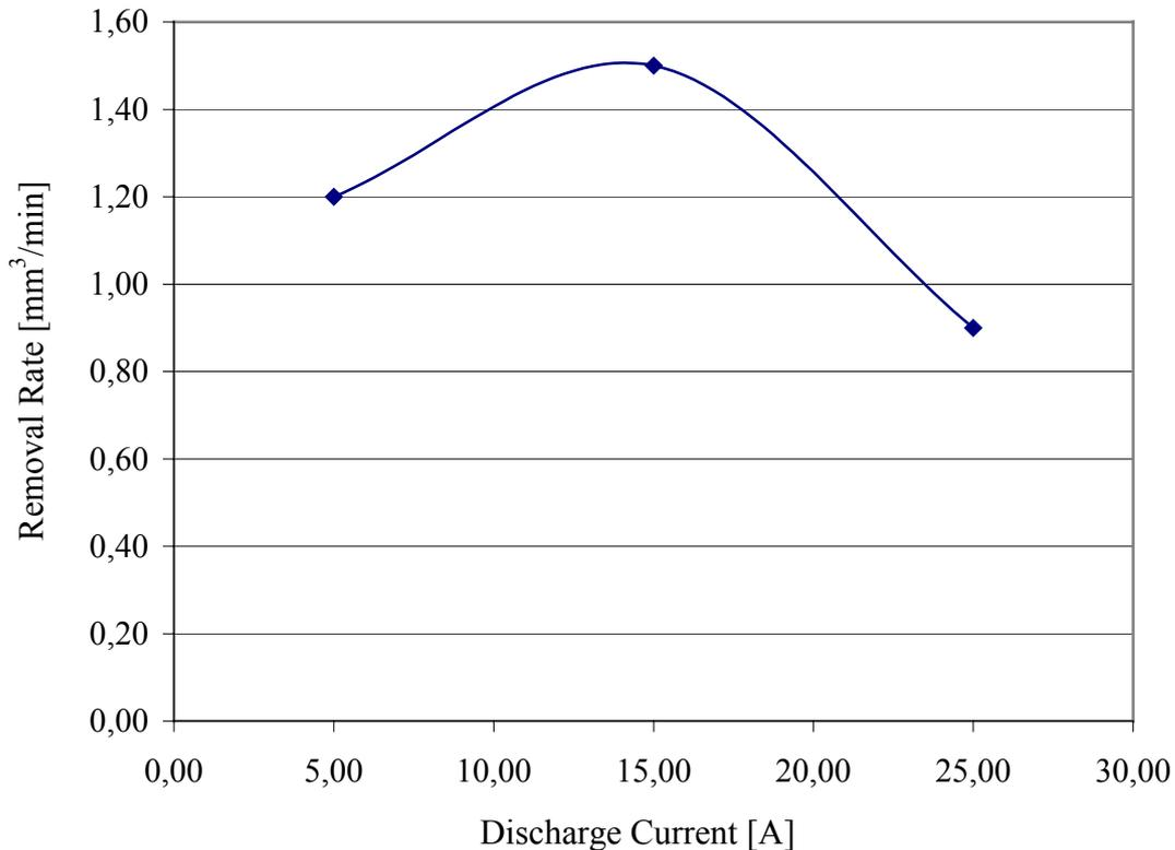
**Figure 1. Removal rates for different discharge durations for TiAl6V4**
