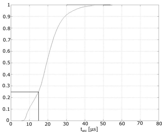
The empirical cumulative distribution function shows for every  $t_{arc}$  value how big is the portion of abnormal discharges showing a  $t_{arc}$  smaller or equal
