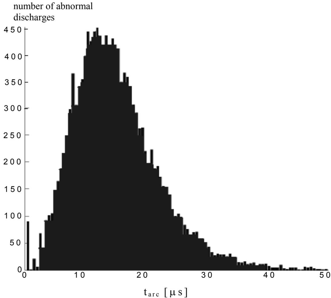
**Figure 5. Histogram of  $t_{arc}$  recorded during extended burning time**
