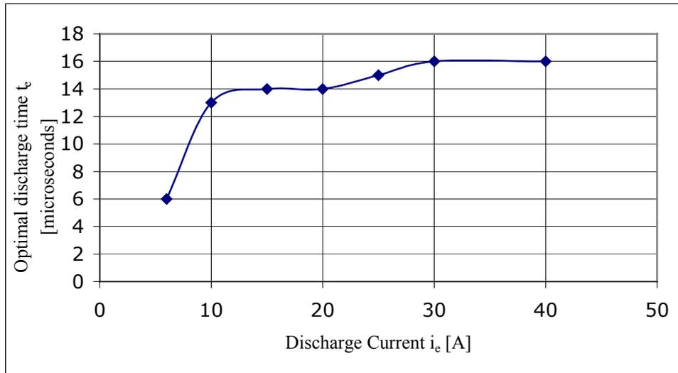
**Figure 8. Identified combinations of  $I_e/t_e$  for TiAl6V4 using  $t_{arc}$  analysis**
