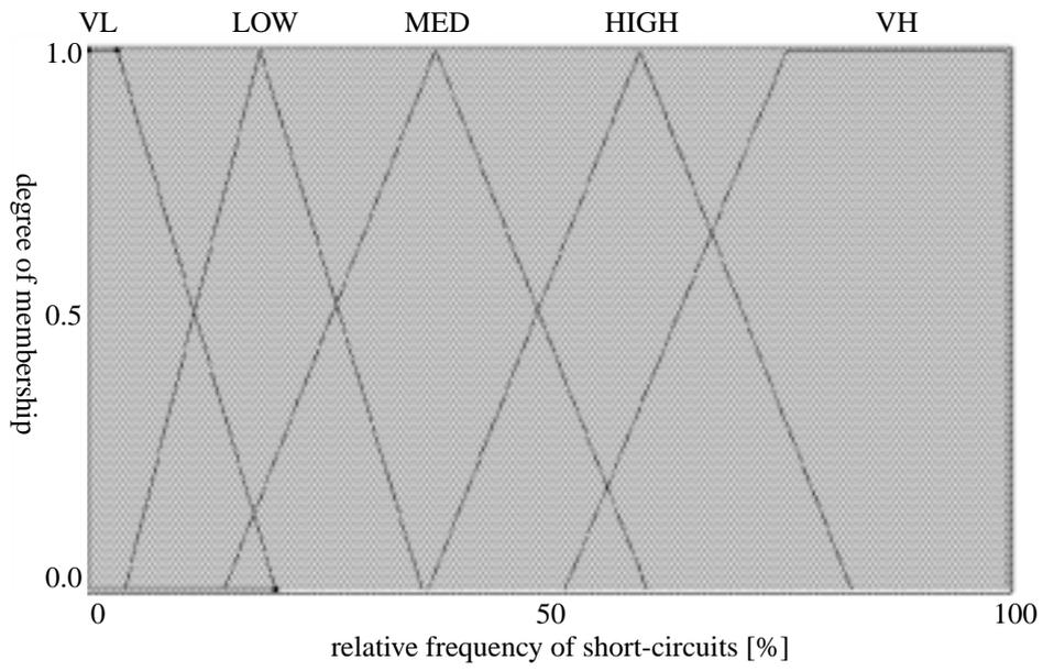
Figure 14: Membership-functions of the input „relative frequency of short-circuits“
