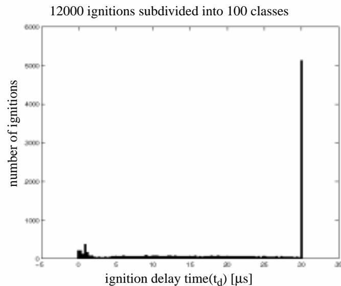
Figure 10: Histogram of ignitions recorded during the ED-process using the SC/OC-controller
