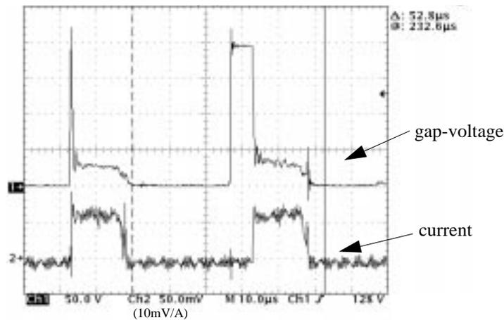
Figure 2: Hard rise of gap-voltage at pulse beginning
