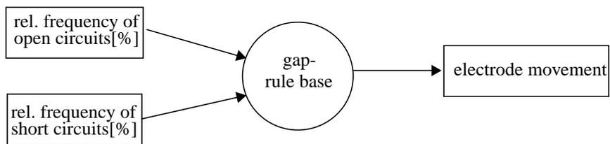
Figure 12: Fuzzy-architecture of the SC/OC-based gap-width controller
