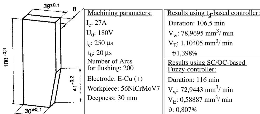
Figure 18: EDM-sinking of a wedge shaped electrode
