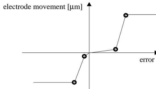
Figure 4: Characteristic function of the  $t_d$ -based controller
