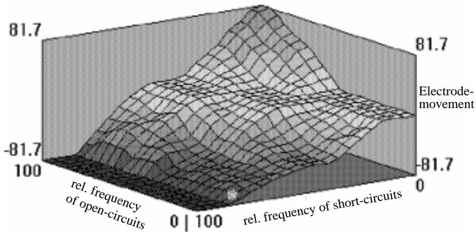
Figure 16: Illustration of gap-width controller function in 3-D
