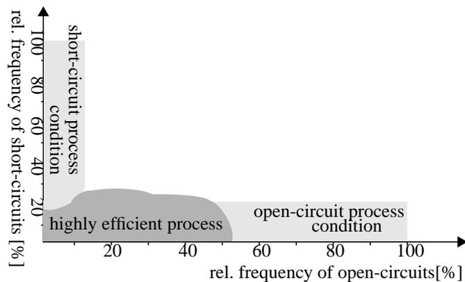
Figure 3: Different process conditions characterized by the relative frequency of short-circuit and open-circuits
