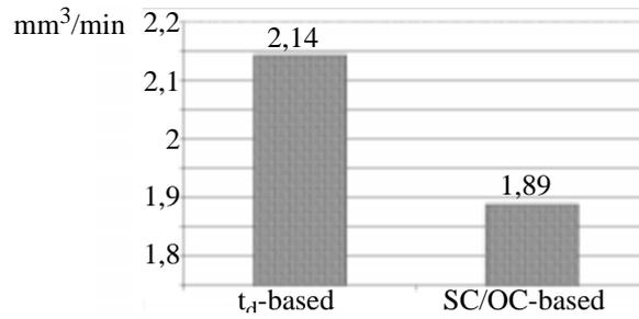
Figure 7: Electrode wear for roughing application
