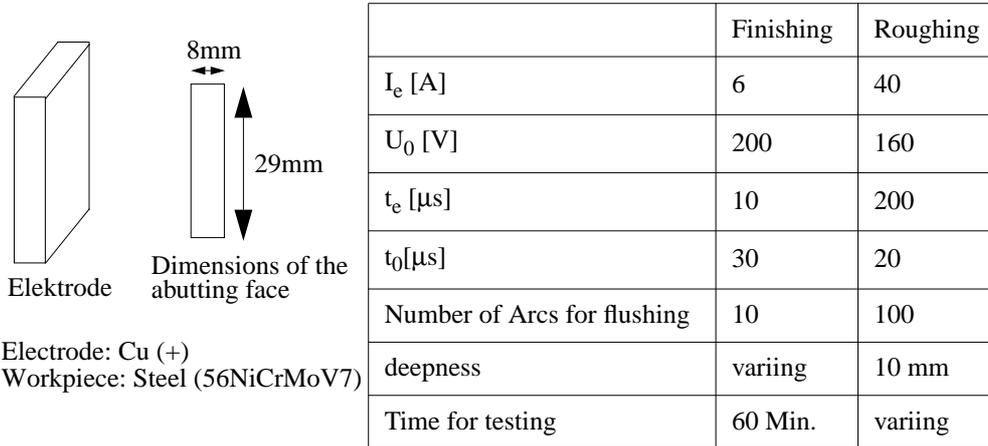
Figure 5: Machining parameters and electrode geometry used for comparison of the different gap-width controllers.
