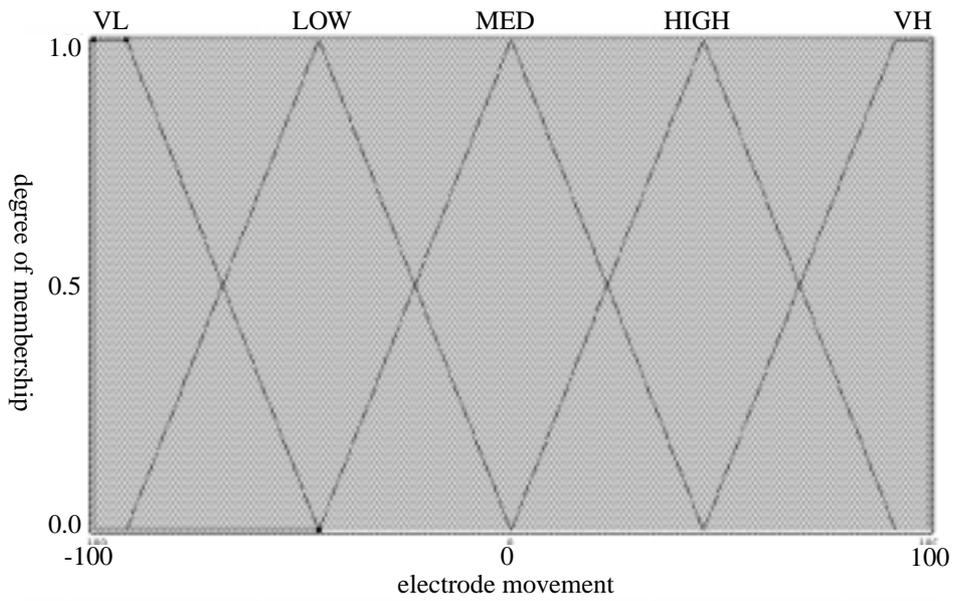
Figure 15: Membership-functions of the output „electrode movement“
