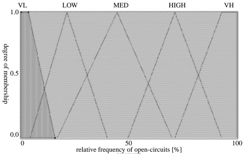
Figure 13: Membership-functions of the input „relative frequency of open-circuits“
