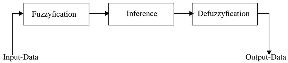
Figure 11: Principle design of a fuzzy control system [17]
