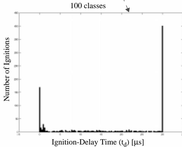
**Note:** Due to the engaged generator technology all pulses which did not show an ignition after 30 μs are classified as open-circuits and switched off. As a consequence open-circuits can be found in the histogram by an ignition delay time of 30 μs.
